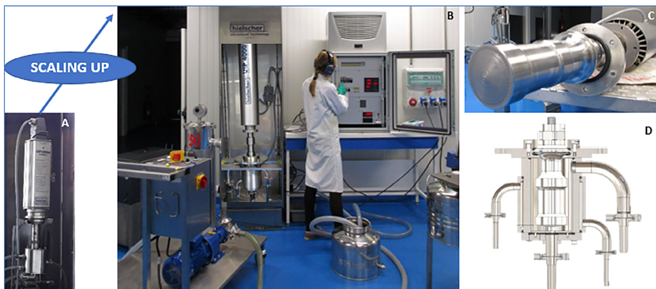
Fig. 9. Scaling up of manothermosonication: from laboratory equipment (A) to pilot scale equipment (B, C & D). On picture D is schematized a transversal section of the US chamber.
