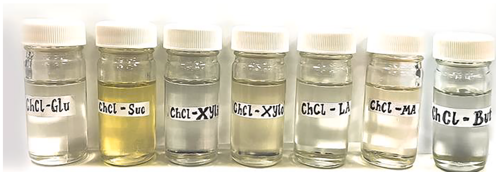
Fig. 2. The various NADES used in this study. From the left to right: Choline chloride-Glucose ( \text{ChCl-Glu} ), Choline chloride -Sucrose ( \text{ChCl-Suc} ), Choline chloride-Xylitol ( \text{ChCl-Xyli} ), Choline chloride-Xylose ( \text{ChCl-Xylo} ), Choline chloride-Lactic acid ( \text{ChCl-LA} ), Choline chloride-Malic acid ( \text{ChCl-MA} ), choline-1,4 Butanediol ( \text{ChCl-But} ).
